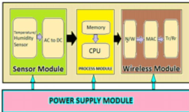
Figure 1: Various components of a sensor node
